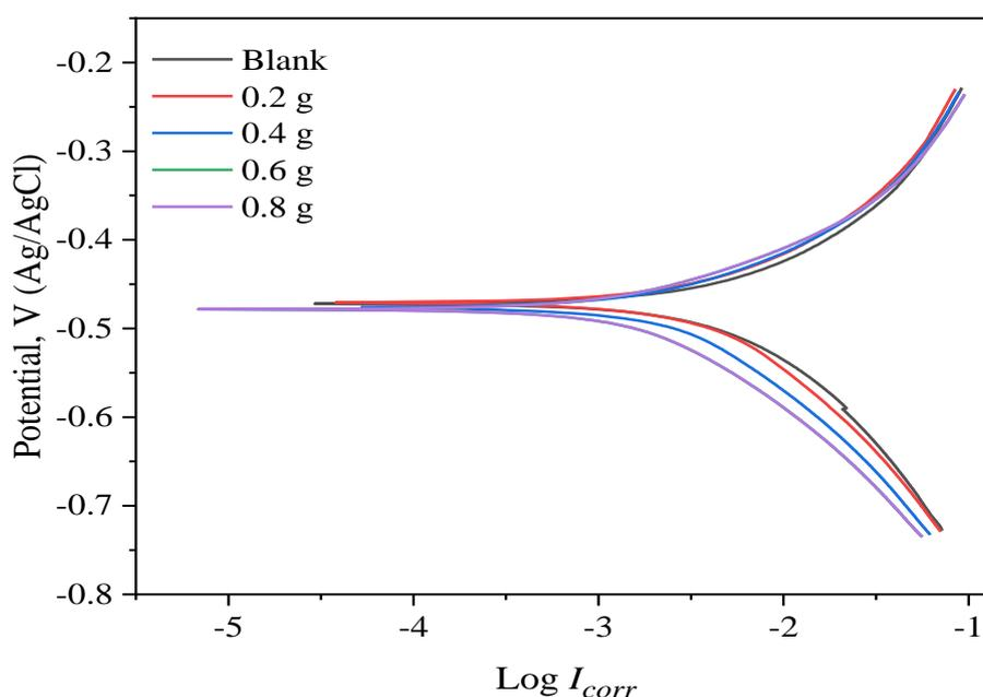
Fig. 5. Potentiodynamic polarization curves for mild steel in various concentration with and without (TG) dye.
