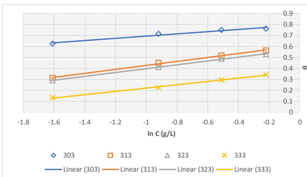
**Fig. 13. Temkin adsorption isotherm of TG Dye for mild steel in 1 M HCl solution in different concentration of TG dye**
