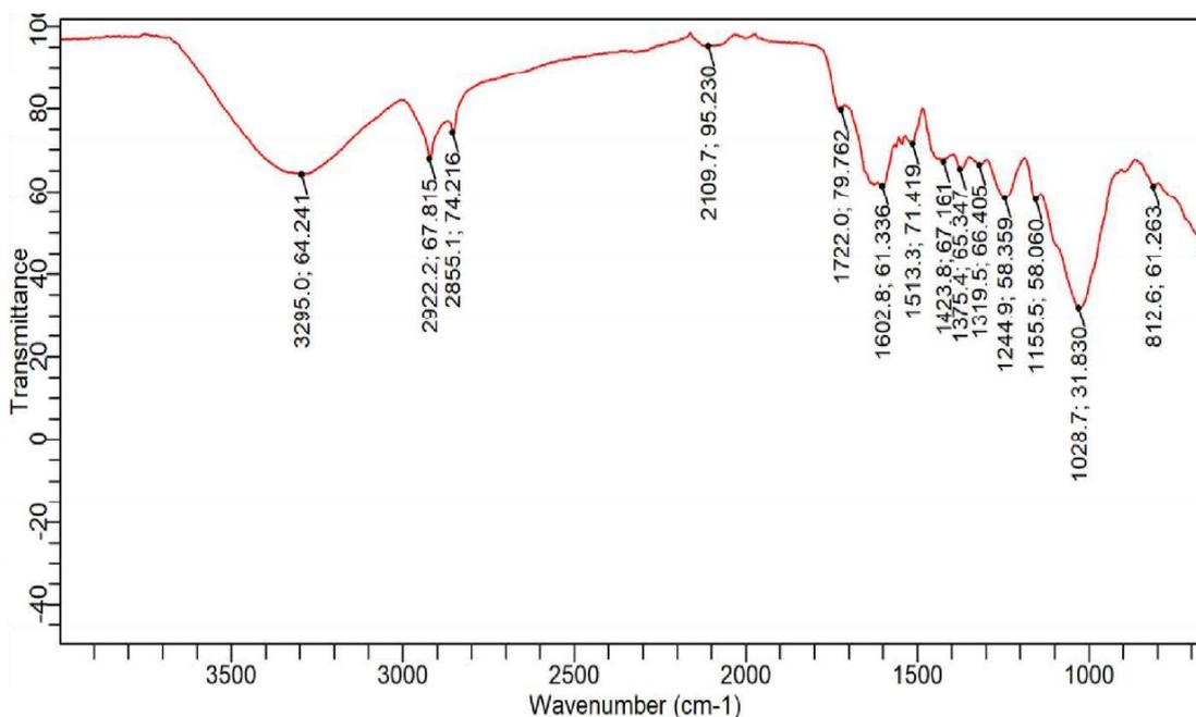
Fig. 2. FTIR spectrum of TG dye
