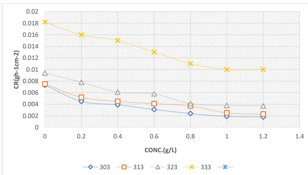
Fig. 3. Effect of TG dye on corrosion rate
