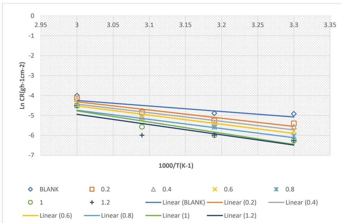
Fig. 9. Relationship between ln CR and 1/T for mild steel in 1 M HCl solution in different concentration of TG dye
