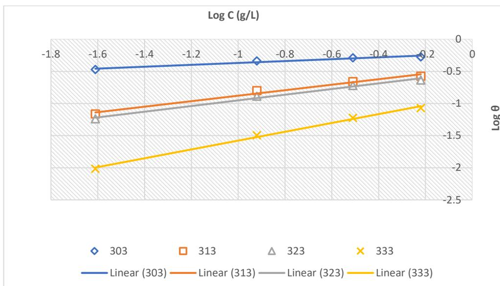
**Fig. 12. Freundlich adsorption isotherm of TG Dye for mild steel in 1 M HCl solution in different concentration n of TG dye**
