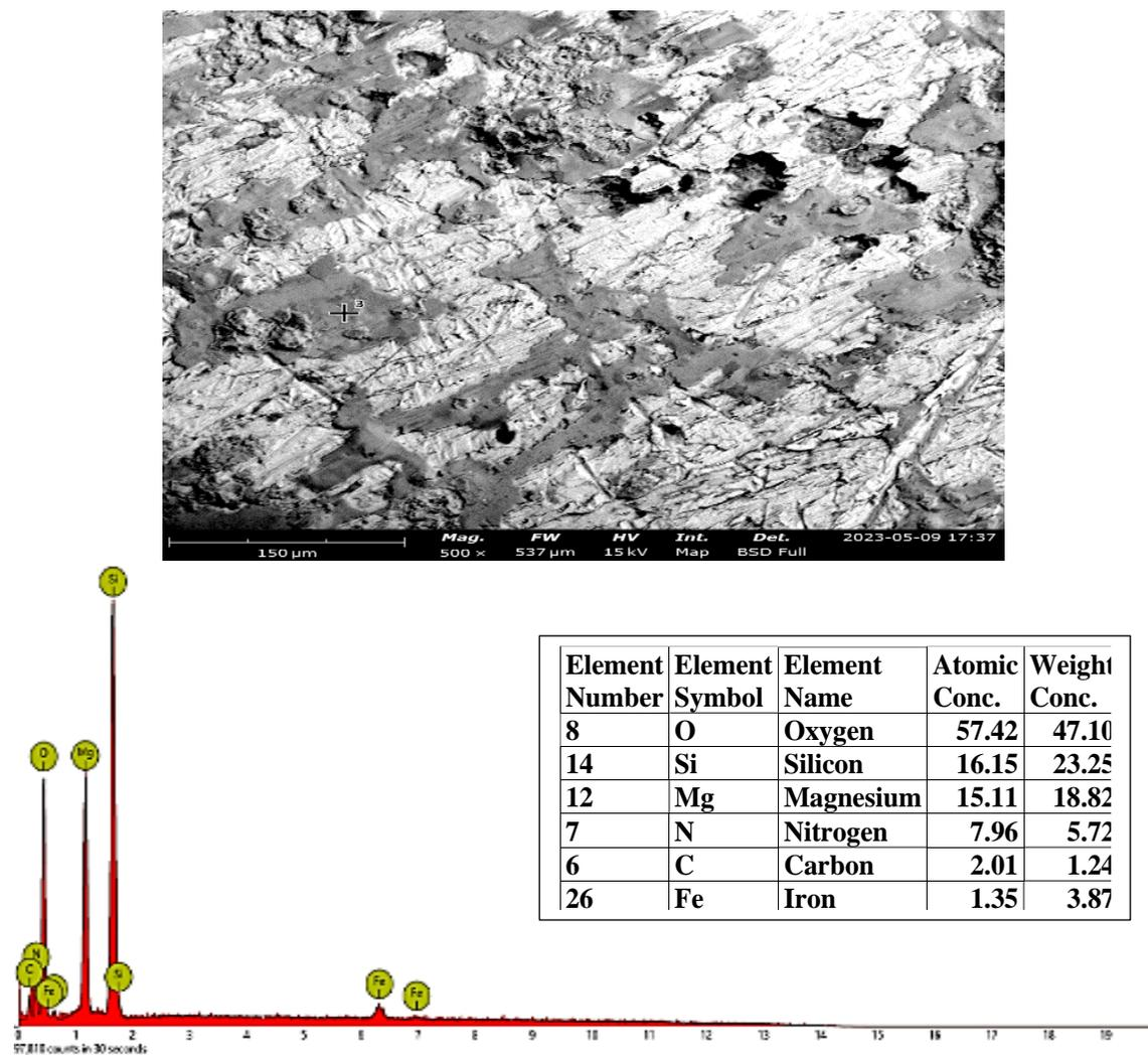
Fig. 14(b). SEM image and EDX analysis of mild steel after immersion in 1M HCl Blank solution
