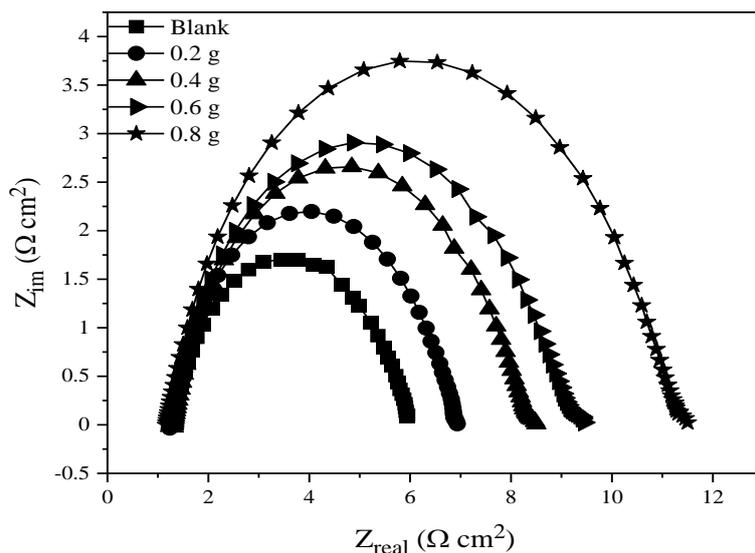
Fig. 6. Nyquist plots for mild steel corrosion in 1M HCl with and without (TG) dye
