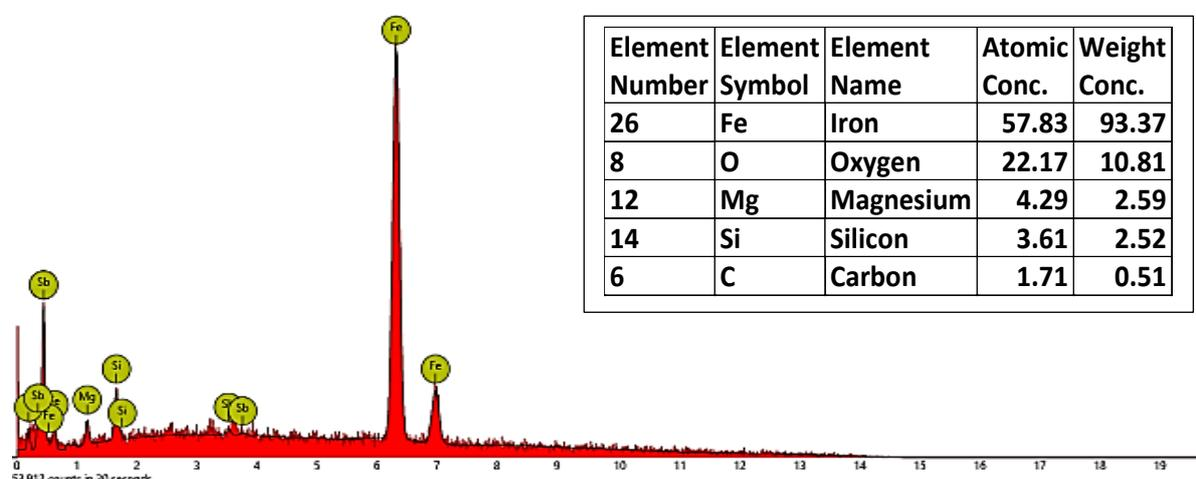
**Fig. 14(a). SEM image and EDX analysis of mild steel**
