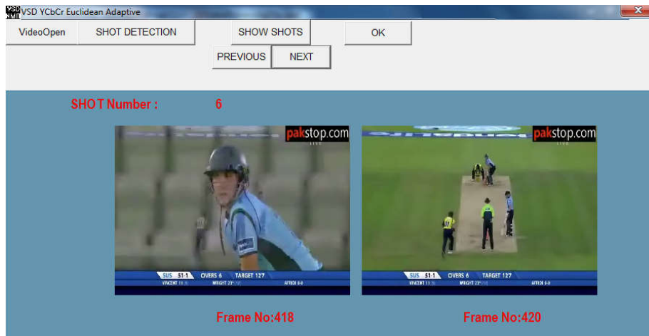
Fig. 4. Detection of shots with frames of before detection and after detection
