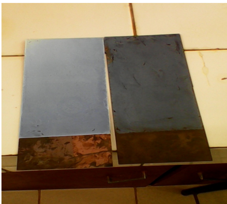
Thin layer of TiO 2 P25 onto stainless steel after annealing at 450 °C for 1 h
