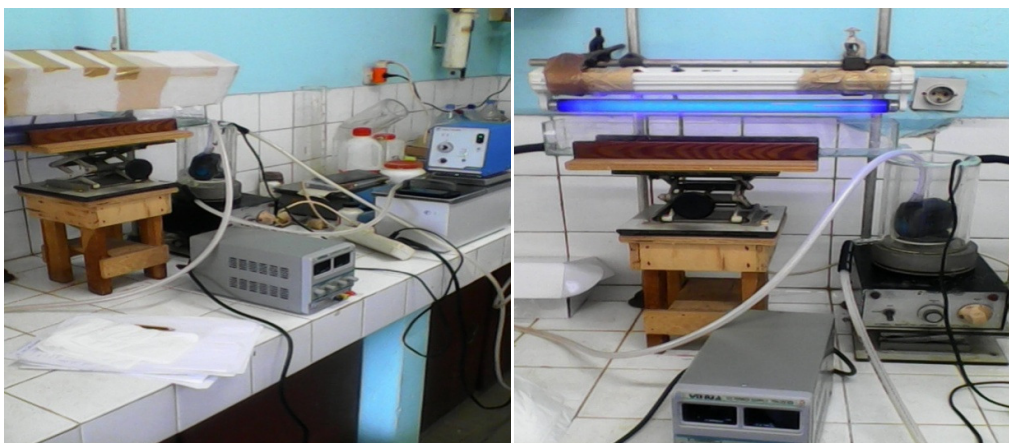
Reactor used for catechol and hydroquinone removal by photooxidation
