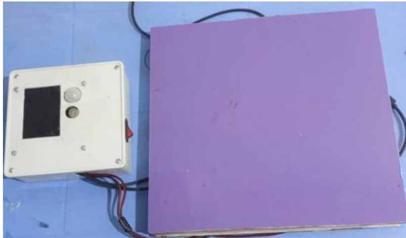
Fig. 7. Hardware of the gas gauging system
