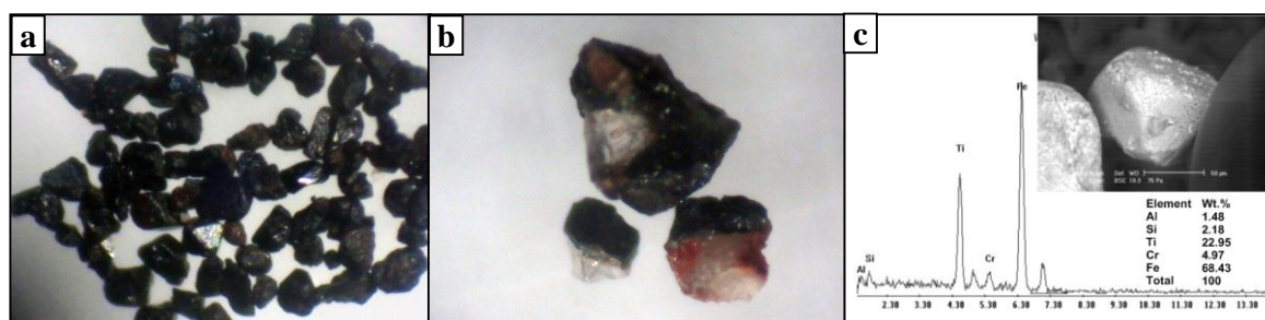
Figure (7): Photomicrographs show aggregates of magnetite and composite grains of magnetite and quartz (a&b), X35, EDX and BSE image of titanomagnetite grain (c).
