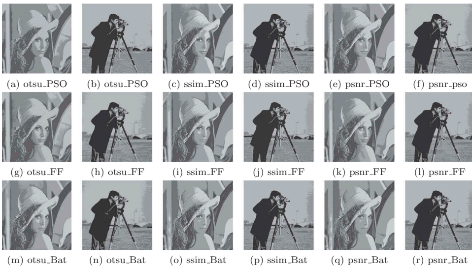
Figure 4. 3_ level thresholding for lena and cameraman images according to the thresholds obtained by the different objective functions using PSO, FF and Bat algorithms.
