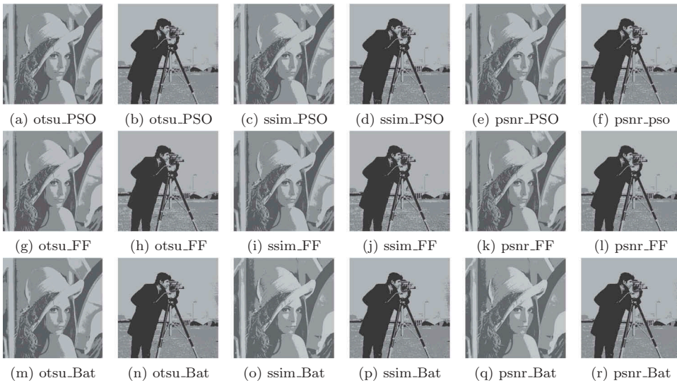
Figure 3. 2_ level thresholding for lena and cameraman images according to the thresholds obtained by the different objective functions using PSO, FF and Bat algorithms.
